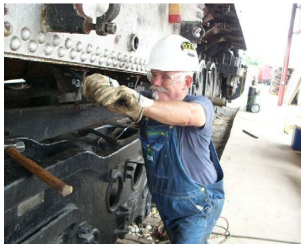
Top: NSPS President Shane Meador cuts the seams in preparation for boiler tube removal.
